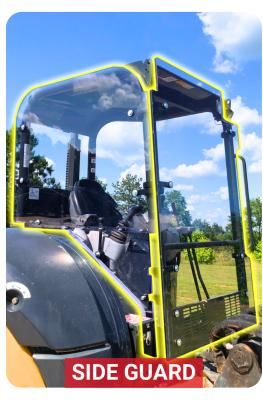
Available for mini size excavators only with an open cab. Side guard is optional.
